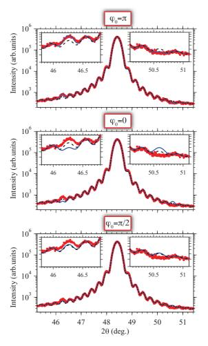
FIG. 6. (Color online) X-ray-diffraction scan of the Cr film cooled to 20 K (red points). A fit using Eq. (A4) assuming a displacement free lattice  $A_{\rm SW}=0$  (black dashed line) and a SW  $A_{\rm SW}>0$  (blue solid line) with a varying phase of the SW with respect to the substrate-Cr interface. The amplitude and period of the SW are fixed. The data are consistent with  $\phi_0=\pi$ , which is described in the main text [see Fig. 2(a) of the main text].
