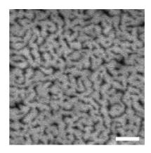
FIG. 8. Scanning electron microscopy (SEM) image of the sample. The scale bar shows 200 nm.
