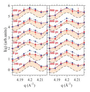
FIG. 4. (Color online) X-ray-diffraction scans for different time delays of the excited (laser on, red circles) and ground state (laser off, blue squares). Data for different delays are shifted vertically for better visibility. The black dashed line shows the intensity without CDW obtained from the fit in Fig. 2(a) and corrected for the effective temperature (see below). The shaded region indicates the area corresponding to the CDW for different delay times.
