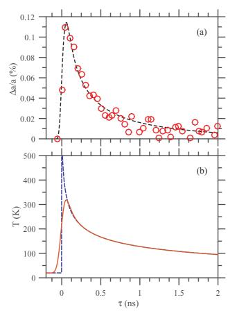
FIG. 7. (Color online) (a) The measured lattice expansion (red circles) and the simulation using Eq. (C1) (black dashed line). (b) The calculated temperature of the film before (blue dashed line) and after (red solid line) convolution with a Gaussian function (100 ps FWHM), representing smearing by the x-ray pulse.
