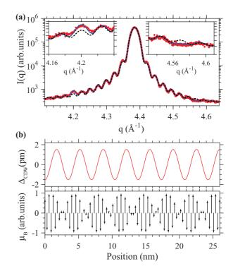
FIG. 2. (Color online) (a) X-ray-diffraction scan of the Cr film cooled to 20 K (red circles) and theoretical fits with CDW (blue solid line) and without CDW (black dashed line) taken into account. Insets show enlarged regions of the diffraction scan. (b) Displacement  $\Delta_{CDW}$  (top) consistent with the x-ray-diffraction data in (a). The magnetic moment  $\mu_B$  (bottom) was inferred from the phase relation between the CDW and SDW [21]. The interface with the substrate is at position 0.
